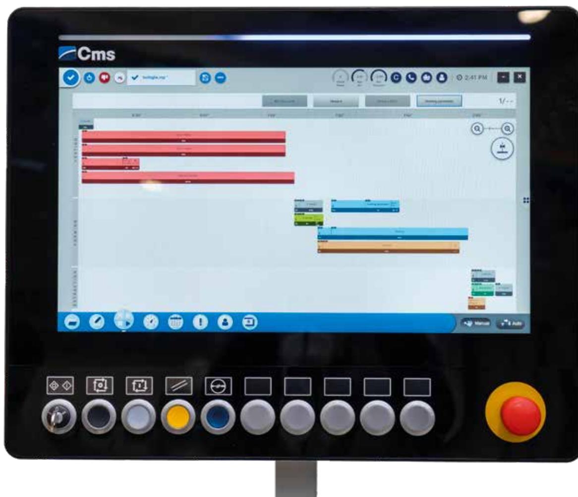
New CMS HMI Thermo Active software designed specifically for the thermoforming process. The timeline and exclusive dashboard make supervising production and the process control instant and easily understandable.
