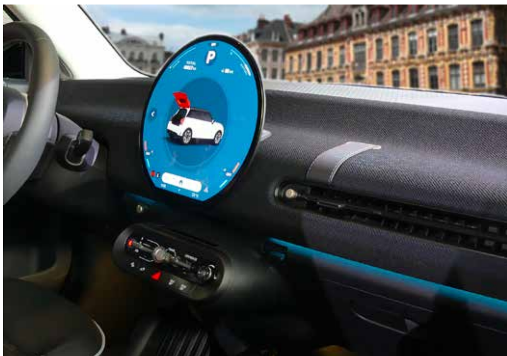
The instrument panel carrier (IP carrier) of the Mini Cooper E is one of the first applications of TechnoCompound's RTU compounds in vehicle interiors.
