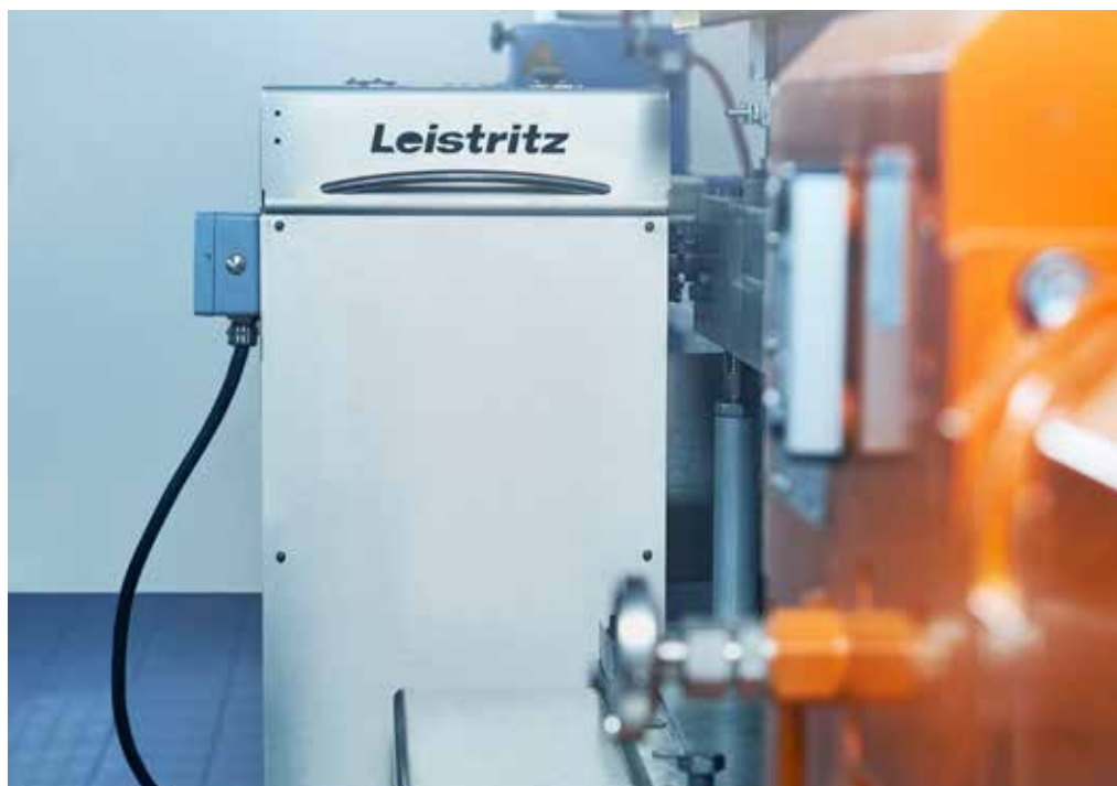
Fig. 2: The Leistritz elongational rheometer continuously determines the melt flow rate during processing to react to fluctuations of the raw material by adding additives - completely without product loss.
