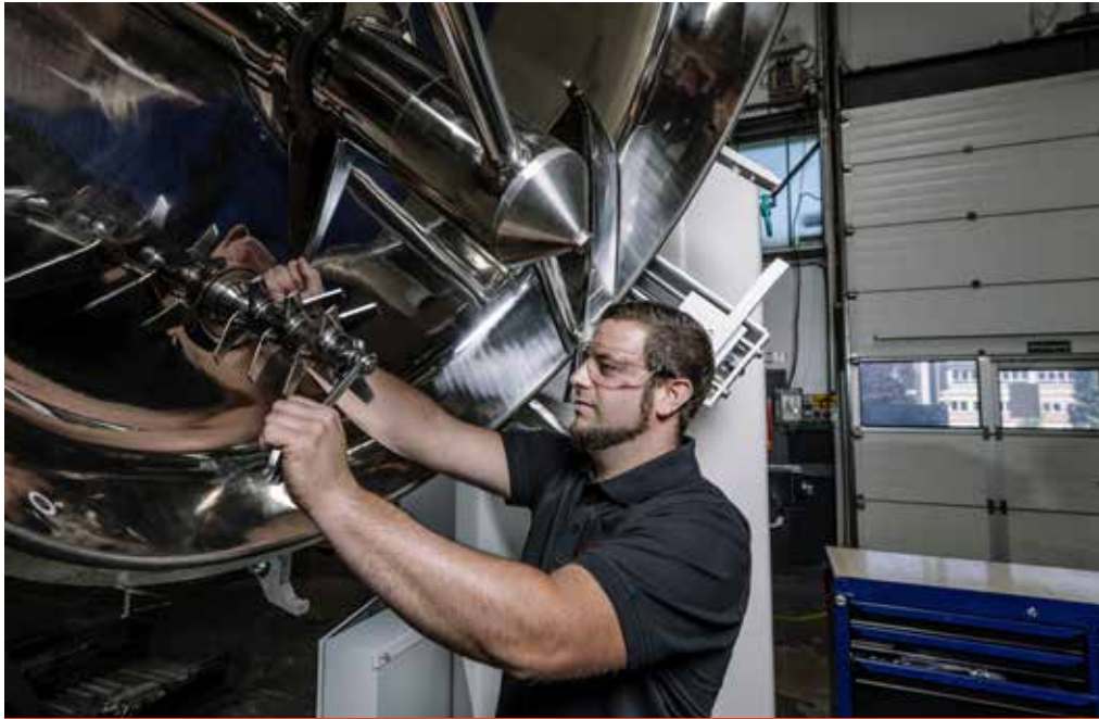
One of MIXACO's Production department member, adjusting one of the tools of the model Container Mixer 2000 Multitool. An innovative and patented technology with multiple mixing motors and new tools enables highly flexible mixing processes of the Multitool™ container mixer. A special arrangement of the mixing tools prevents the materials from heating up and sticking to the tools, the mixing head and the container.
