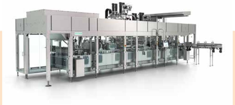
Ampack's innovative tunnel design separates the production area from the mechanical parts to ensure safe filling of sensitive products on the FBL.
